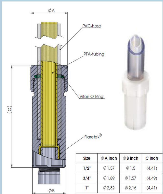
The PFA tubing inside the PVC hose with kink free Flare connection at both ends offers outstanding flexibility and provides ultimate safety!
