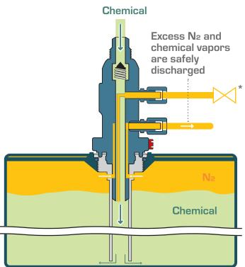
Note: The N<sub>2</sub> connection is a standard flare 1/4" connection. Other versions on request.
